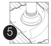
To finish, remove the protective film on the top of the Rapid Flash
